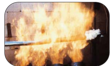
Thorburn's Ball Joint Armor-Flex™ tested at 1100°C
